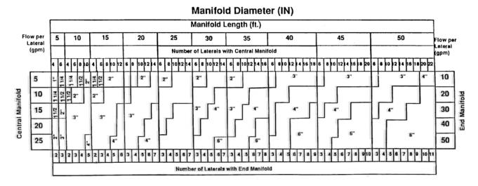
Computed for Plastic Pipe Only. The Hazen-Williams equation was used to compute headlosses through each segment (Hazen-Williams C<sub>h</sub>-150). The maximum manifold length for a given lateral discharge rate and spacing was defined as that length at which the difference between the heads at the distal and supply ends of the manifold exceeded 10 percent of the head at the distal end.
